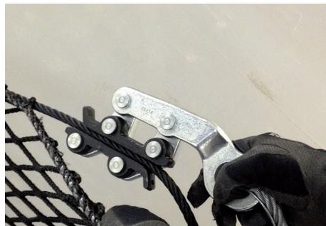
**g.** (1 person) Set the telescoping rod for the upper wire pulley in the stay closest to the anchor point.
